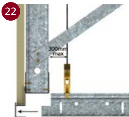
■ VERTICAL SCREW-FIX SYSTEM DETAIL
