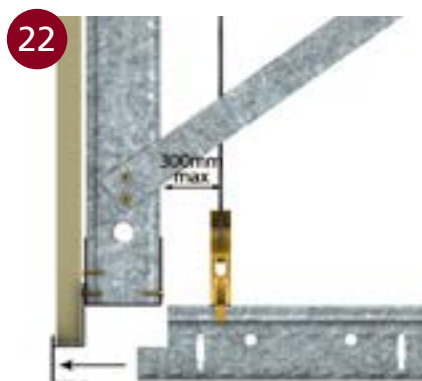
■ VERTICAL SCREW-FIX SYSTEM DETAIL
