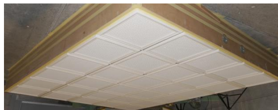
Test specimen installed for testing (image inverted to depict ceiling installation)
